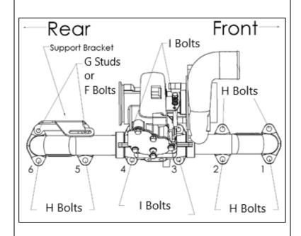
Install the support bracket on the top two rear bolts (cylinders 5 & 6) using either two **G** studs and two **N** nuts or the two **F** bolts provided depending on your installation. Position four of the **P** washers between the manifold and the bracket as shown in the picture.
