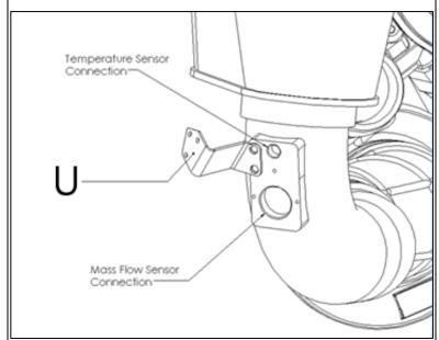
40. Install the factory temperature sensors into the ports using the provided S and T bolts. On some trucks the wires may be very tight. It is very rare but, if wires are too tight it may be necessary to lengthen the wires by splicing in small segments of wire. It is best to solder the wires together and cover with wire shrink tubing. These ports are placed in the only location on the tube which yields the proper flow speed of the air, for the mass air flow sensor to read properly.
