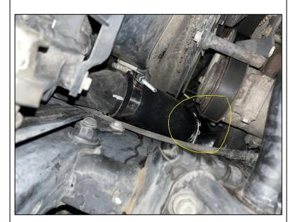
Note: If it is difficult to slide couplers on, you can use a small amount of soapy water to help the charge pipe slide into the couplers. DO NOT USE OIL TO DO THIS as oil will not dry and the charge pipe may slip out under pressure.
