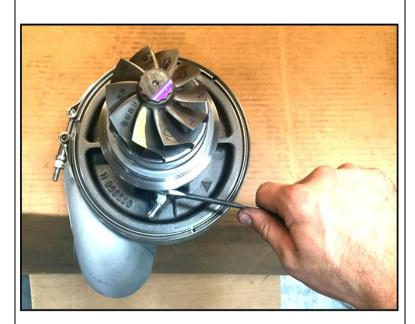
30. Install oil supply line (steel braided hose without elbows) to the oil inlet elbow fitting on large turbo as shown. Tighten the fitting snug, but do not over tighten.
