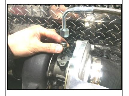
22. Lastly, attach the other end of the steel braided hose to the factory oil feed from the truck.
