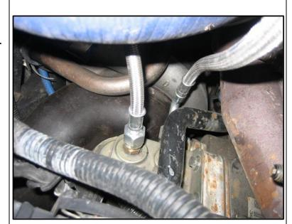
Connect the shorter oil drain line to the large turbo using two **K** bolts and the last **D** gasket provided in the kit.
