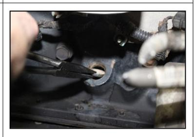
Remove the rear factory oil 17. drain from the block. Insert the provided long oil drain line into the front drain port and short oil drain line in the rear hole (where factory drain line was connected). Keep drain lines as straight as possible while pushing them into the holes, so you do not damage them. Make sure they are pushed completely into the hole. Both O-rings should be inside the hole. The long oil drain line will be connected to the top turbo later as shown.
