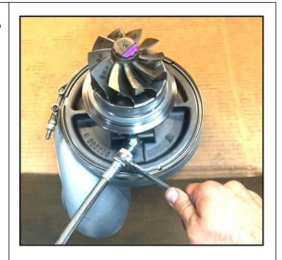
31. Carefully lower the large turbo section to the front of the turbine housing installed in the truck and insert the turbine wheel into the turbine housing. Do not allow the exposed turbine fins to touch anything. They can easily be damaged. Use v-band clamp to secure the center section in place but keep it slightly lose to allow adjustment. Orient the bearing housing so the oil supply port faces up and oil drain port points down (vertical of each
