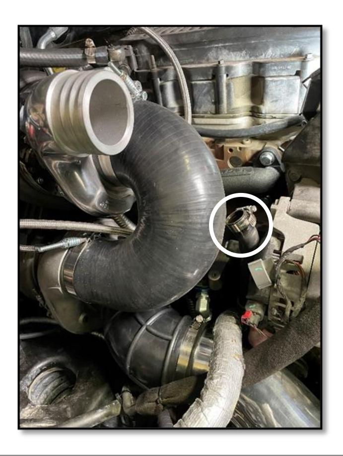
14. Reroute the Riser to the firewall heater core. Plug the line going into the top on the engine block.
