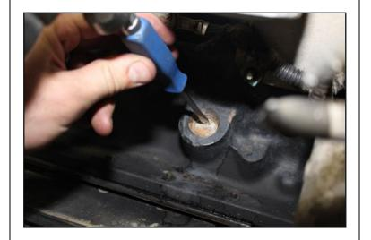
NOTE: Be sure to clean around the freeze plug and remove all debris from the cup of the freeze plug to make sure nothing drops into the oil pan. Be very careful not to push the plug into the oil pan, or you will have to drop the oil pan to retrieve it.
