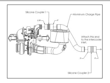
Note: If the charge pipe does not line up with the intercooler inlet, you may need to rotate the small compressor housing slightly. To do so, loosen the 8 bolts that hold the housing just loose enough that the housing can rotate but not rattle. Rotate the housing to where it needs to be, then re-tighten all 8 bolts. Aluminum thread can be striped easily. Only tighten to appx. 10 ft.lbs.
