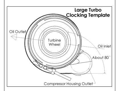
29. Install the oil inlet elbow fitting provided in the kit. Tighten it so the fitting points toward the compressor outlet side as shown.
