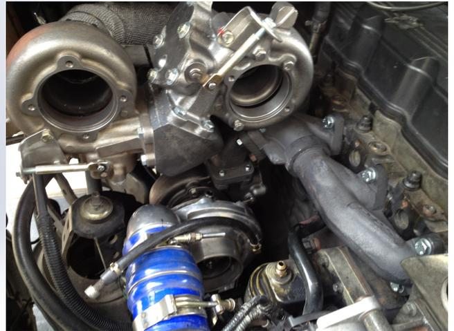
6. Insert the turbo cartridges into the exhaust housings, starting with the lower turbo. Attach the oil drain and oil supply lines to the turbos. Tighten the four turbine bolts with the little brackets to secure. Then attach the wastegate hose to the fitting on the compressor housing. The lower turbo wastegates off exhaust pressure. The spring gate has been pre-set, but can be adjusted later (shorter=more boost). We recommend driving it first before adjusting it.
