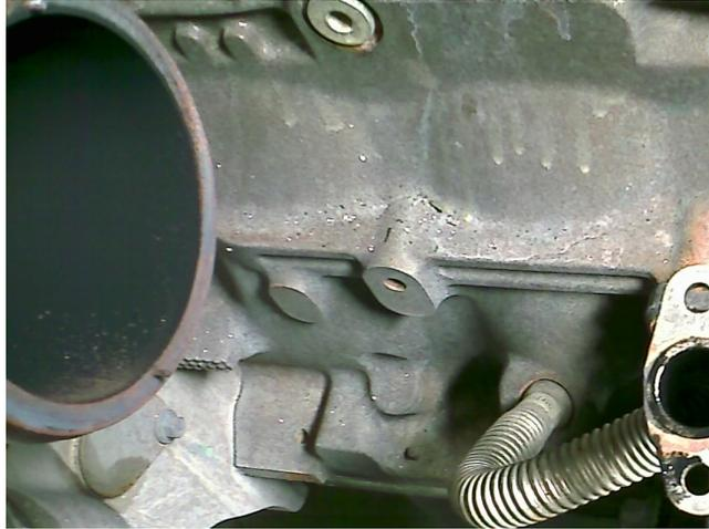
Next. Locate the front or rear freeze plug (same height as the other oil drain port). Take a punch or screwdriver and lightly tap on one edge of the freeze plug to get it to rotate or twist inside the hole. Then take a pair of needle nose pliers and remove the freeze plug (BE VERY CAREFUL NOT TO PUSH THE PLUG INTO THE OIL PAN, OR YOU WILL HAVE TO DROP THE OIL PAN TO RETRIEVE IT).
