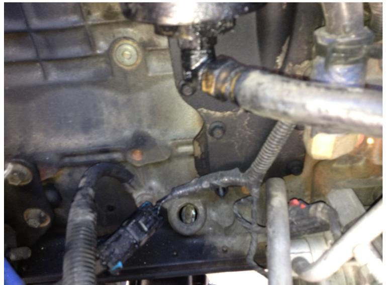
Next take the provided oil drain fitting, and push into the front oil hole.
