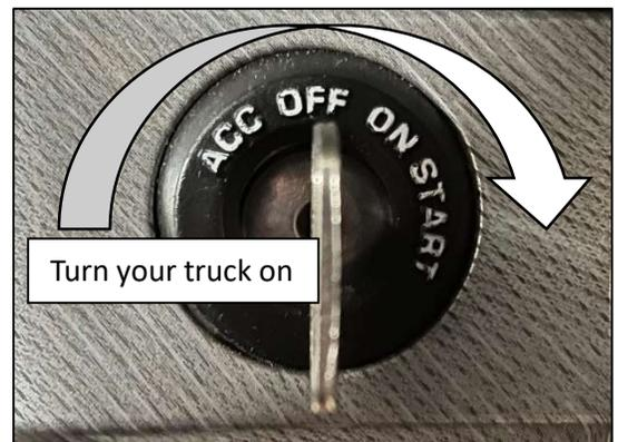
**Step #2:** Locate the “Starting Position” variable within the data logger. This variable displays the state of the starting position dial located in the cab of your truck. Test that this variable changes from 1 to 11 as you change the position of the dial.
