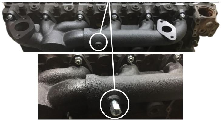
After installation, drive truck for approximately 100 miles then, while the truck is warm re-torque all the manifold and turbo bolts, as the bolts sometimes loosen up after being heated and cooled a few times.
